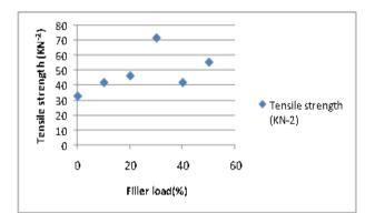
Figure 3. Effect of filler loading on tensile strength of flexible polyether foam
