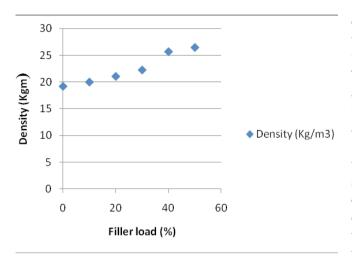
Figure 1. Effect of filler load on Density.
