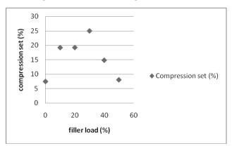
Figure 2. Effect of filler loading on compression set of flexible polyether foam
