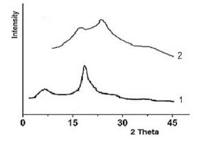
Figure 2. X-ray diffractograms for samples of CS (1) and PC (2)
