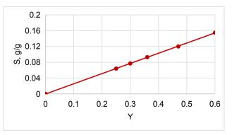
**Figure 10.** Dependence of sorption value at  $\varphi$ =0.7 on amorphicity degree of cellulose samples
