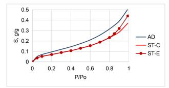
Figure 7. Calculated isotherms of WV for AD of C6P (AD) and sample of semicrystalline ST (ST-C); ST-E is experimental isotherm of ST sample
