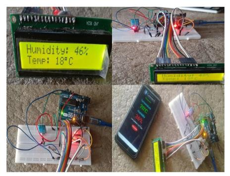
Figure 9. Wireless Temperature & Humidity Monitoring System
