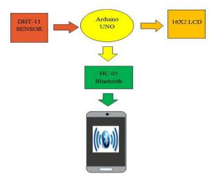
Figure 1. Block Diagram of wireless real time Temperature and Humidity monitoring system
